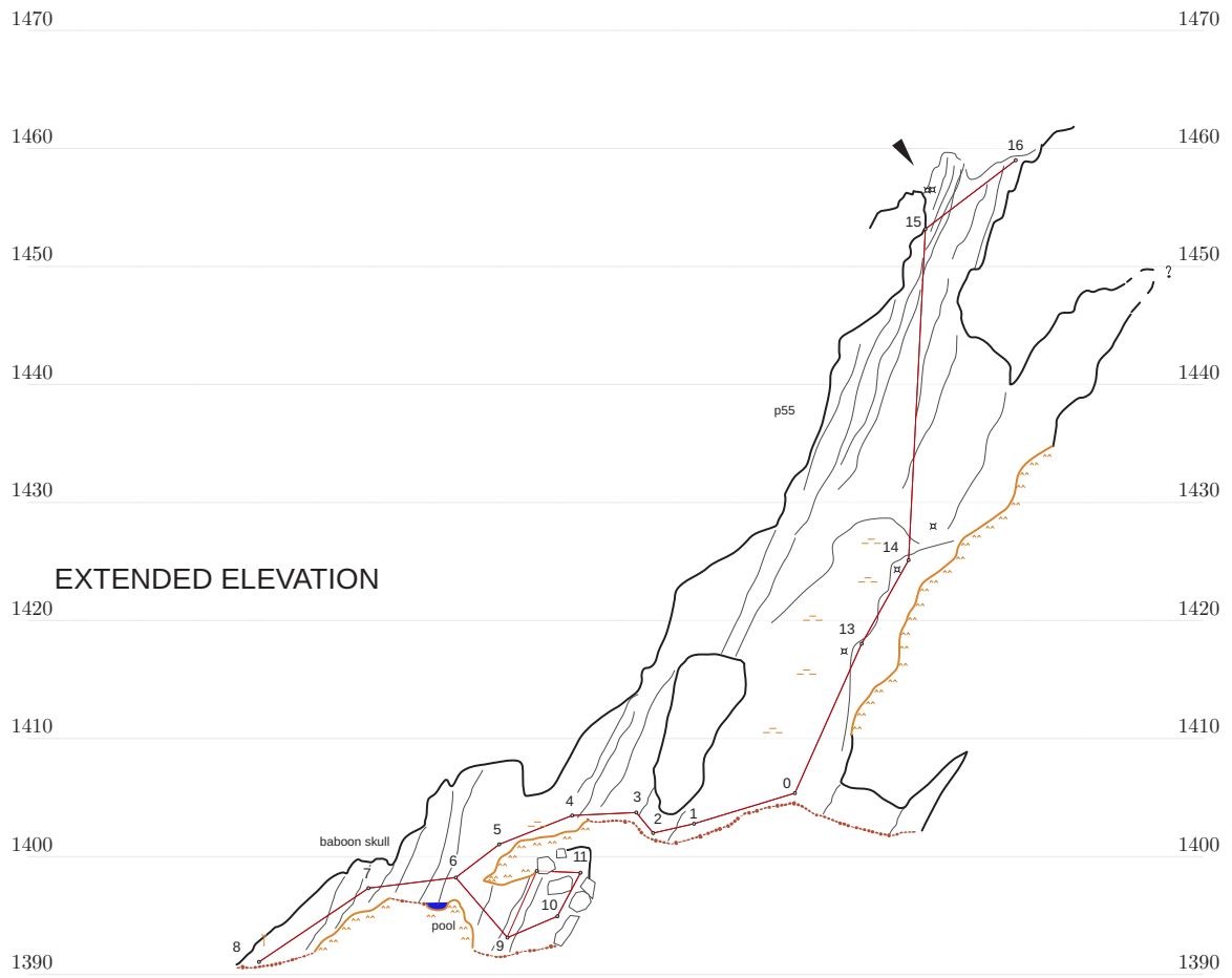
Extended elevation of Starling Shaft (scaled)
